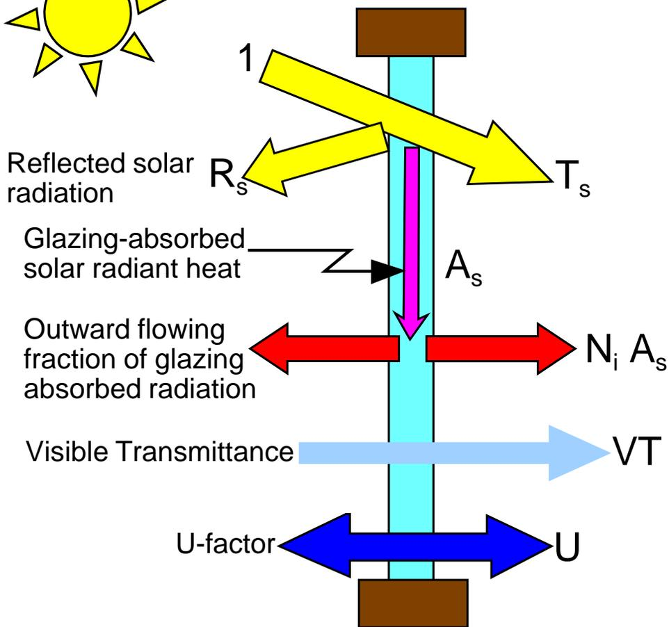
Solar Heat Gain Coefficient
