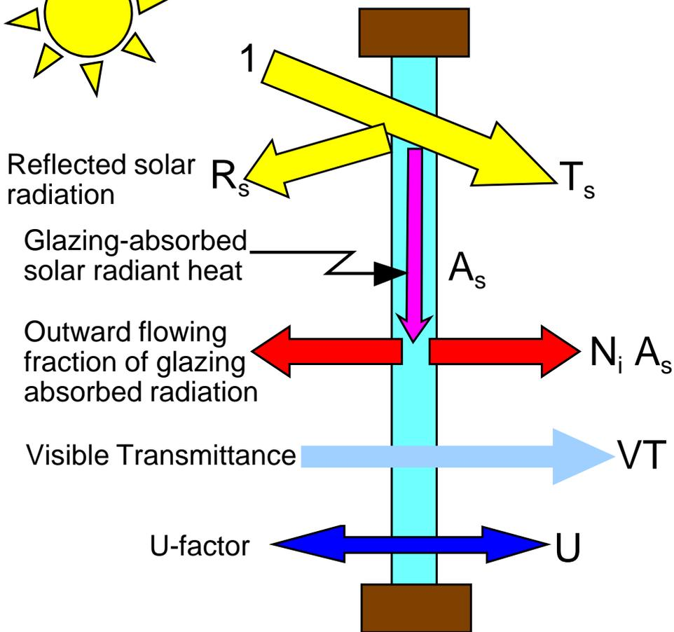
Solar Heat Gain Coefficient
