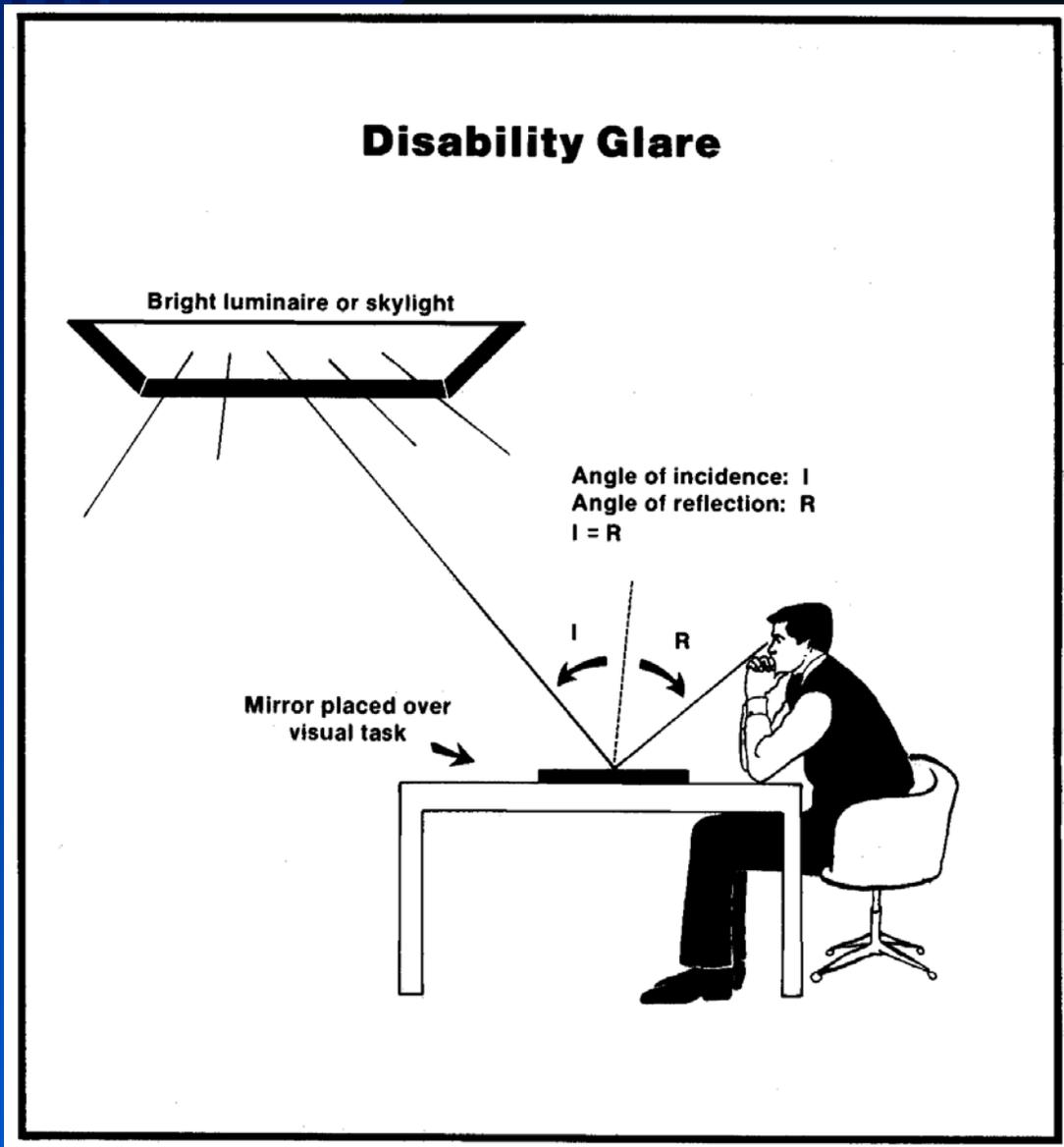
Light from overhead or behind you reflects from a shiny task. The reflected light is so bright as to greatly reduce the contrast of the task, making black letters, for example, almost as bright as the white page surrounding them. The result is a “veiling” of the task, a washing out or masking of the target, thereby disabling your ability to see the task. This is why it is called disability glare.
