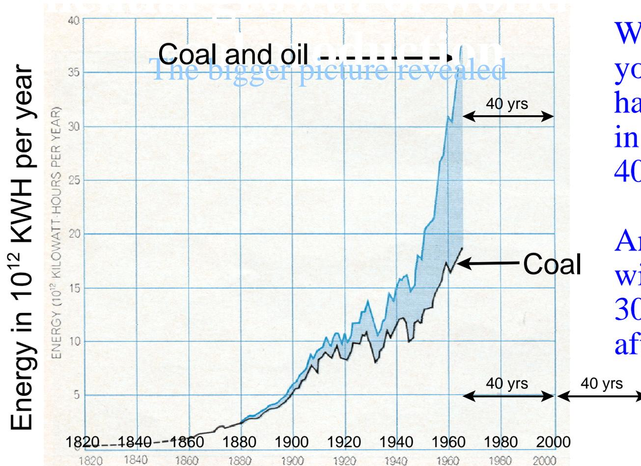
ENERGY CONTRIBUTION of coal (*black*) and coal plus oil (*color*) is portrayed in terms of their heat of combustion. Before 1900 the energy contribution from oil was barely significant. Since then the contribution from oil (*shaded area*) has risen much more rapidly than that from coal. By 1968 oil represented about 60 percent of the total. If the energy from natural gas were included, petroleum would account for about 70 percent of the total.
